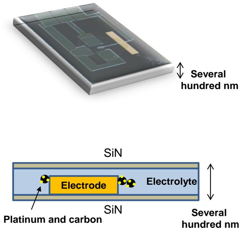
Using micro-electromechanical systems technology to create microscopic electrochemical cells that can be observed via transmission electron microscope
