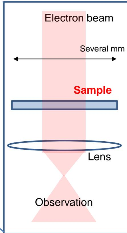
**Requirements for observation by transmission electron microscope**
