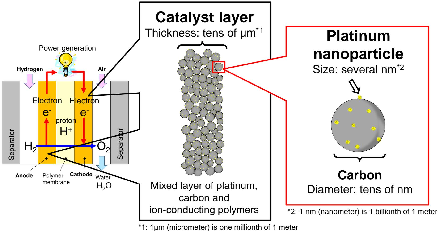
Anodes and cathodes are primarily composed of platinum nanoparticles and carbon
