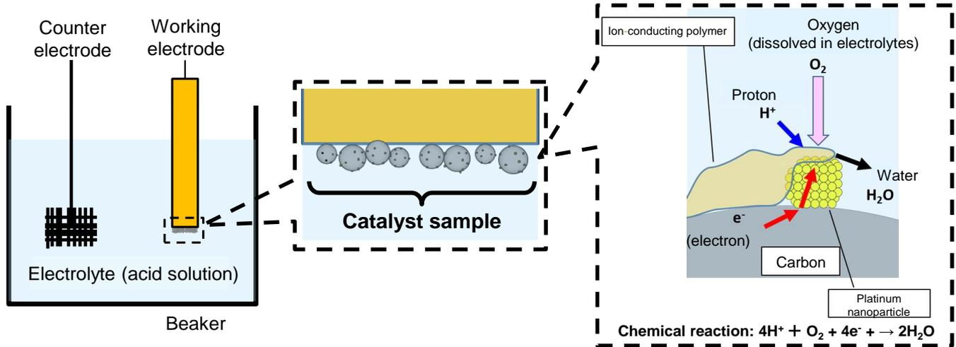
The conventional technique uses the general catalyst evaluation method to reproduce the chemical reactions that occur in fuel cells
