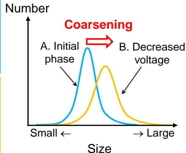
Conventional technology compares platinum nanoparticle size during the initial phase and after voltage is decreased
