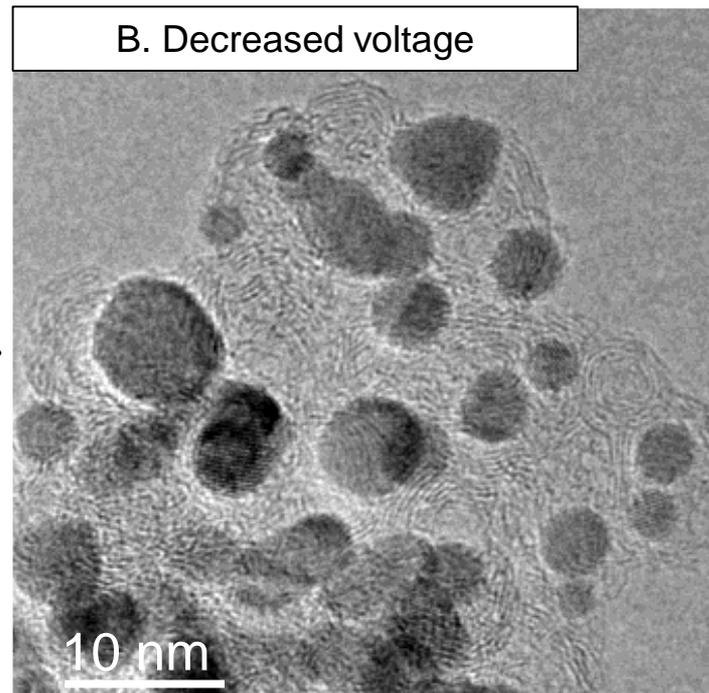
The process of platinum nanoparticle coarsening cannot be fully understood using conventional techniques
