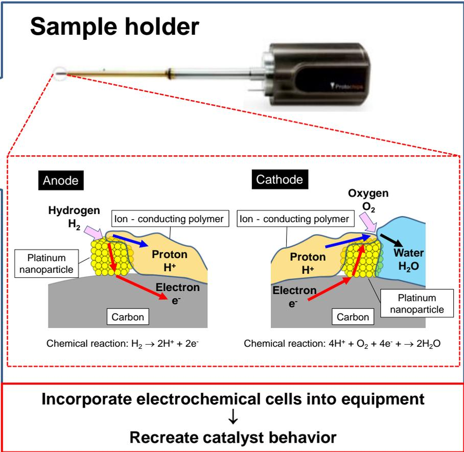
Recreate a fuel cell catalyst chemical reaction in a transmission electron microscope
